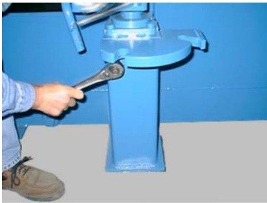
Fig. 2 - 23: Tighten the Mounting Bolts
