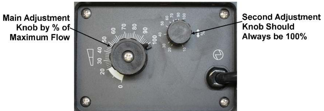
Fig. 4 – 5: Rinse Injector Pump Controls
