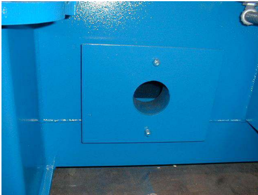
Fig. 2 - 4: Mounting the Combustion Burner (Up to 180,000 BTU)
