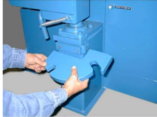
Fig. 2 - 22: Positioning the Door Lock Plate
