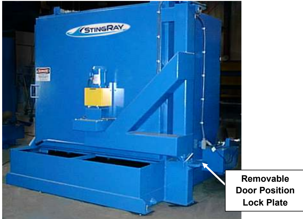
Fig. 2 – 19: Removable Door Position Lock Plate
