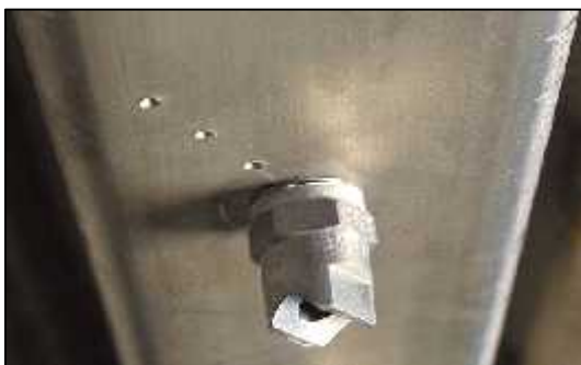
Fig. 1: Cleaning and Replacing the Power Blast Manifold Nozzles
