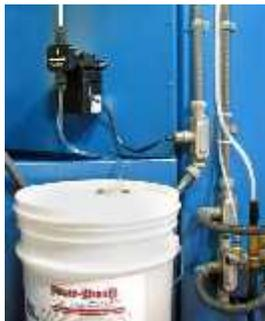
equipped with a rinse inhibitor pump, one can easily be retro-fit.
