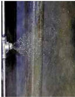
The STINGRAY optional rust inhibitor injection pump mixes a measured amount of [Power Kleen](#) rust inhibitor directly in the rinse water during a rinse cycle. A control allows accurate adjustment of the flow rate. Rust Inhibitor prevents flash rusting and provides short term rust protection for your cleaned parts. If your washer is not
