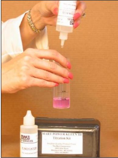
4. Add the acid (verify the percent for your Power Kleen Detergent in the chart below), and count the drops while swirling the sample solution until the pink color is completely gone. Remember to hold the acid bottle vertically when adding drops to ensure consistent droplet size.
