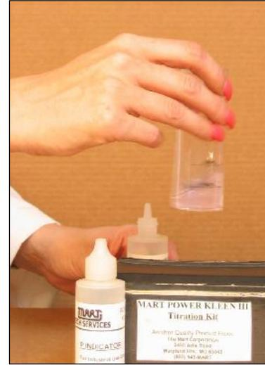
5. Reading: Use the chart below to find the “titration number” for your particular Power Kleen chemical. Divide your “drop count” by the titration number to calculate the oz/gal of concentration.
